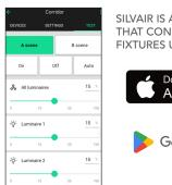
SILVAIR IS A SOFTWARE AND COMMISSIONING APP THAT CONNECTS AND CONTROLS LIGHTING FIXTURES USING BLUETOOTH MESH TECHNOLOGY.
